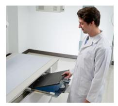
The Precision 600FP system includes a bucky device in the table for digital radiography with the OTS. The bucky is compatible with Konica Minolta AeroDR 14"  $\times$  17" RAD detectors and can be easily switched between landscape and portrait formats by simply rotating the bucky. Switching formats without having to pull out detectors improves workflow, user ergonomics and reduces chances of detector damage.
